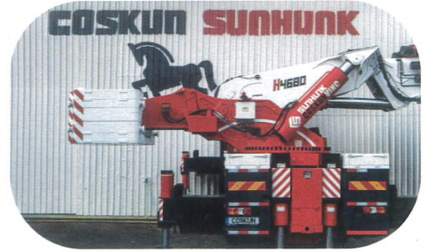
4,50 m tail with 18.000 kg. counterweight
