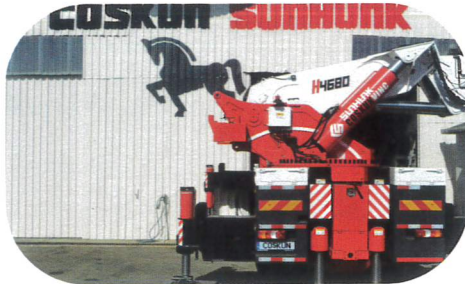
2,25 m tail without counterweight
