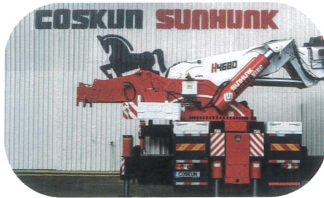
3,80 m tail with 8.500 kg. counterweight
