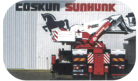
2,65 m tail with 9.500 kg. counterweight
