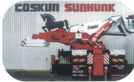
4,50 m tail with 8.500 kg. counterweight
