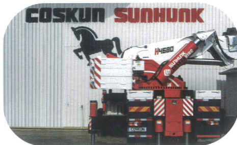
2,65 m tail with 18.000 kg. counterweight
