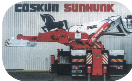
5,50 m tail with 8.500 kg. counterweight
