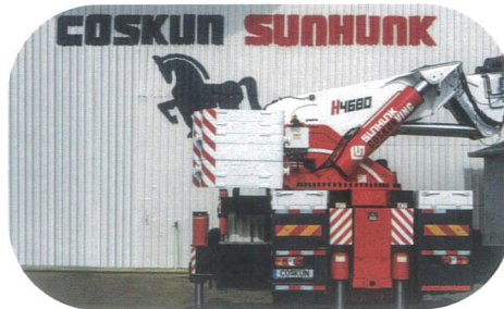
2,65 m tail with 20.600 kg. counterweight
