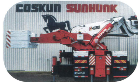
5,50 m tail with 18.000 kg. counterweight
