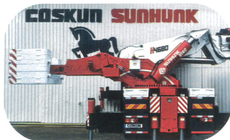
5,50 m tail with 20.600 kg. counterweight
