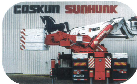
4,50 m tail with 20.600 kg. counterweight
