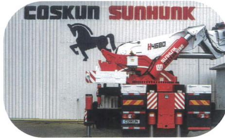
2,65 m tail with 8.500 kg. counterweight
