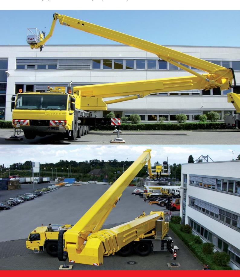
The WT 850 is ideal for the construction, inspection and cleaning of large buildings. A working height of 84 meters basically says it all. Yet the lateral outreach of 30 meters only underscores the platform's great potential. This articulated access platform can be mounted on a standard 48-ton chassis with five axles (3 steerable) chassis. This enables a turn radius of only 14 meters.
